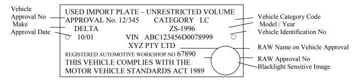
Dimensions 95mm x 35mm (approx) 2 x 3mm holes on horizontal Centre Line
